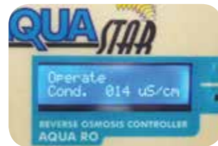
Electric programmer with conductive meter for the control of the quality permeate.
