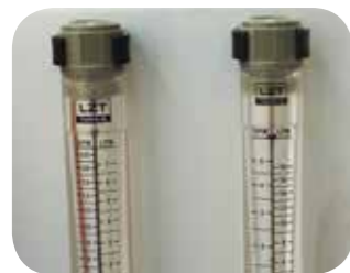
Flow meters reading of concentrated and permeate.
